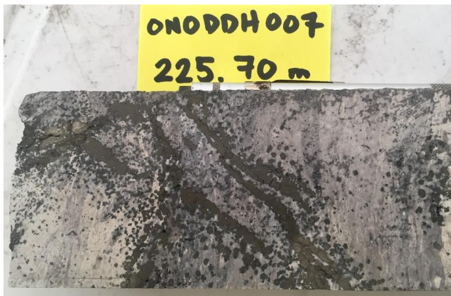
Plate 11 – Altered and mineralized volcanic host rock with up to 7% metallic sulphide in drill hole ONODDH007, HQ core from 225.7 m depth – Ono Island Project, Fiji
