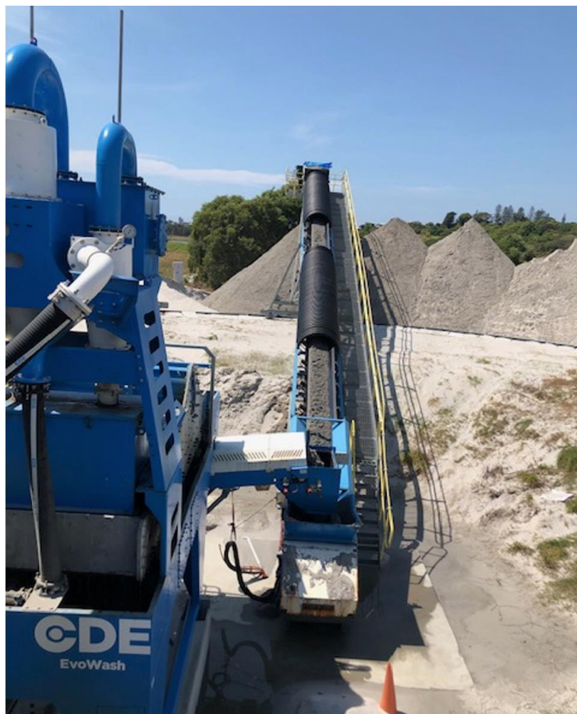
Plate 5 - Dewatered sand stockpiles and mobile stacker
