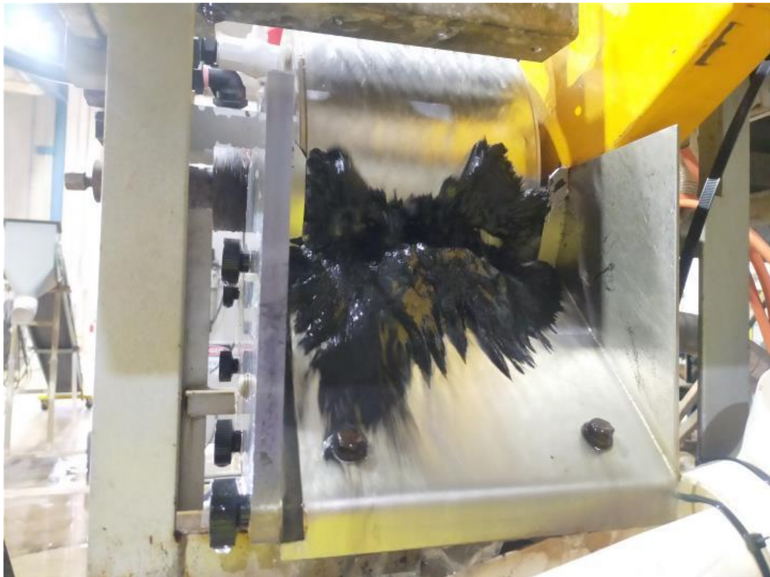
Plate 6 – Magnetite concentrate from large scale pilot plant processing
